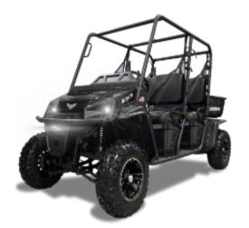
AMP CREW – 4x2 48V CD LITHIUM-ION 5KW/8KW 600 amp controller 30MPH 1,500 lbs 400 lbs
