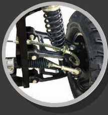
Premium Comfort Suspension Independent Front Suspension with Double Arm
